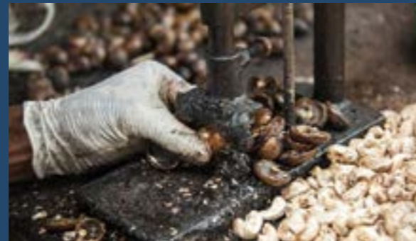
Manual hand operated cashew peeling machine
