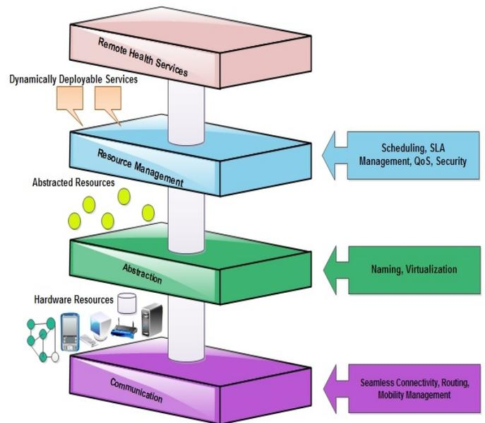
Fig. 1 - A Layered Architecture for Sensor-Cloud Framework
