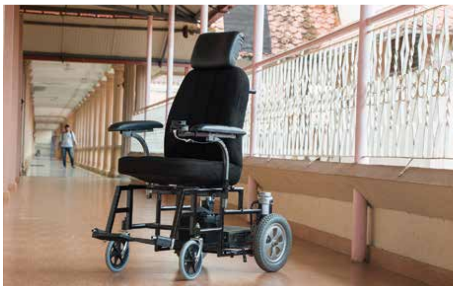
The Self-E wheelchair uses the robotic operating system (ROS) for navigation and allows patients to commute from one place to another. Courtesy of Akhil Raj/HuT Labs/Amrita University.
