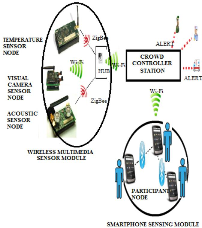
Figure 2. Wireless Sensor Network Architecture for Crowd Disaster Mitigation
