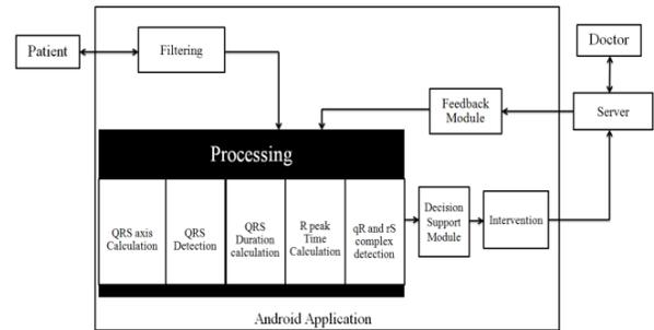
Fig. 1. System architecture showing different modules for the detection and warning of LAHB occurrences.
