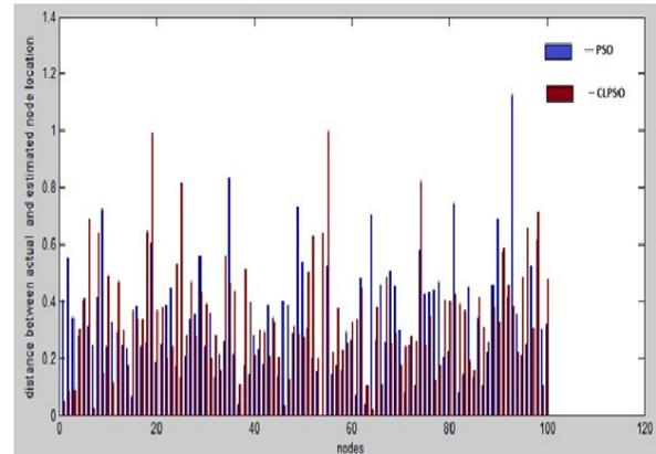
Figure 6: Distance between actual position and estimated position for CLPSO and PSO
