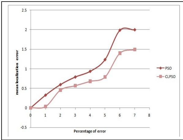
Figure 7: For increasing percentage of error the error rate is observed for PSO and CLPSO
