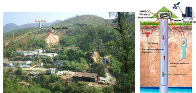
Figure 1: (a) Deployment site in Munnar, Kerala, India, and (b) Intelligent wireless Probe (IWP) with quad sensors
