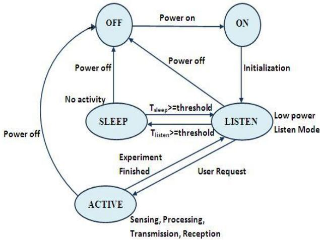
Fig.3. State transition diagram for RT WSN Testbed
