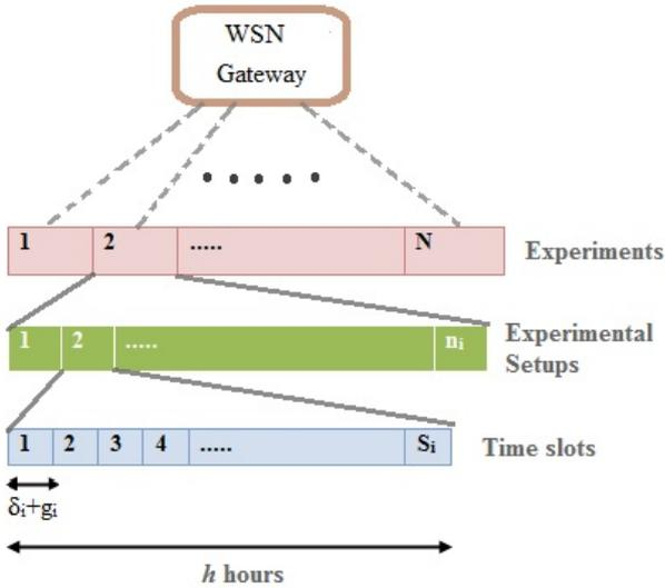
Fig.2. TDMA scheme for RT WSN Testbed
