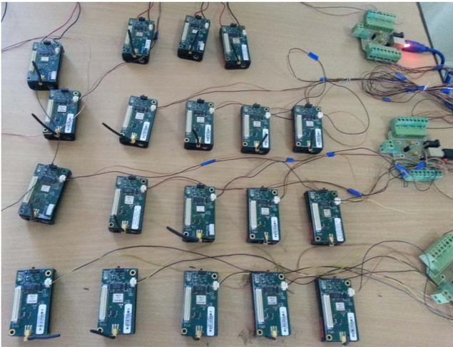
Fig.4. RT Lab WSN testbed
