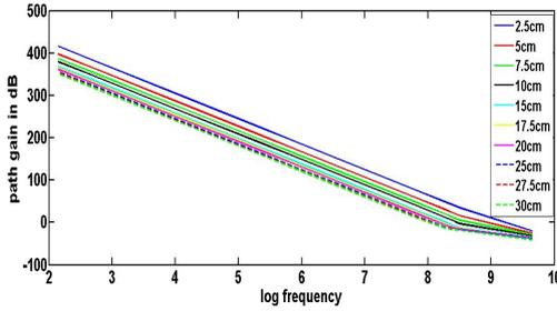
Figure 6: Path Gain vs. Frequency in Muscle
