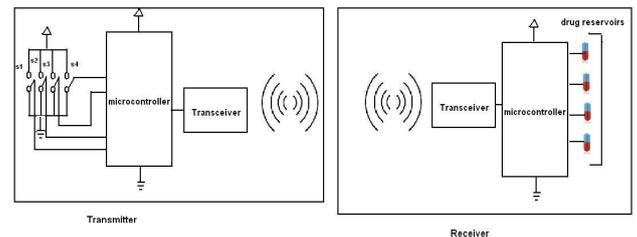
Figure 1: Architecture Diagram for Targeted Drug Delivery
