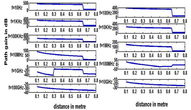
Figure 8: Effect of near field and far field in body and free space
