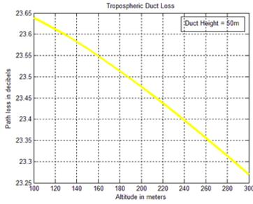
Fig. 5. Tropospheric Ducting Loss
