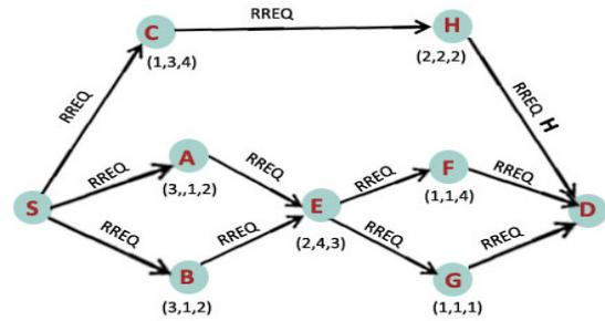
Fig. 1. Tracing Node-Disjoint paths: Node A and B send RREQ to E respectively. E receives and forward only the RREQ from A and rejects the one from B. Destination D receives RREQs from nodes F,G and H. It sends RREPs only to F and H and discards the RREQ from G since it has come from the same neighbor (node A) of the source as has the RREQ from node F. The numbers on each link indicate the signal strength of that link.
