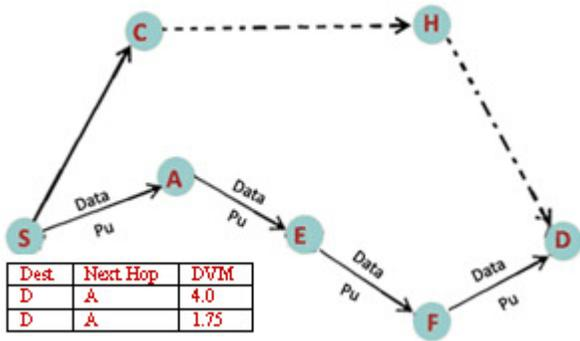
Fig. 4. Source S detects this change through the low DVM. Since the other path now has a higher DVM, source switches its primary path to S-A-E-F-D.
