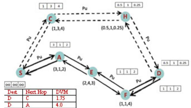
Fig. 3. Suppose node H moves away from nodes C and D. The DVM parameters shows degradation from previous stage. Thus DVM of S-C-H-D become very weak.
