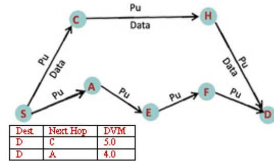
Fig. 2. Source S has received RREPs via two node-disjoint paths: S-A-E-F-D and S-C-H-D. Since path S-C-H-D has a higher Decision Value , it is selected as the primary path. The other path becomes the alternate path. The source sends periodic update(Pu) message periodically along both paths.
