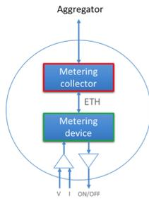
Fig. 2. Metering device showcasing both monitoring and control signal.
