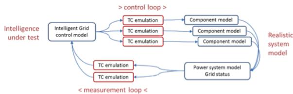
Fig. 6. Emulated communication channels integrated in APROS simulation environment.
