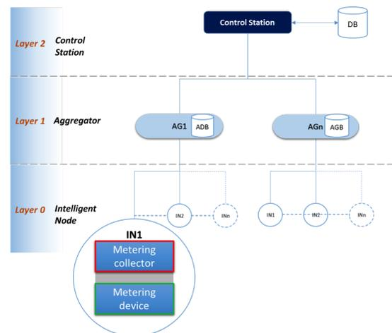
Fig. 4. Hierarchical layout of the test distribution network, showcasing the real-time monitoring and control of physical nodes.
