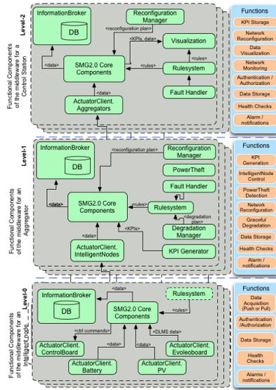
Fig. 5. Component-based architecture of SMG2.0 middleware for hierarchal monitoring and control.
