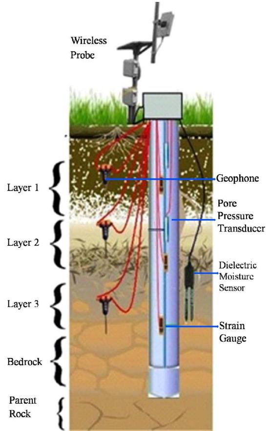
Figure. 4 The new design of DEP with nested geophone assembly. Note the 3C geophone is placed in three sensitive layers.
