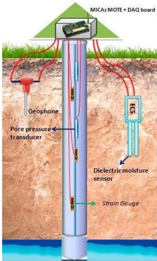
Figure 1. Schematic of Deep Earth Probe (DEP). [1]
