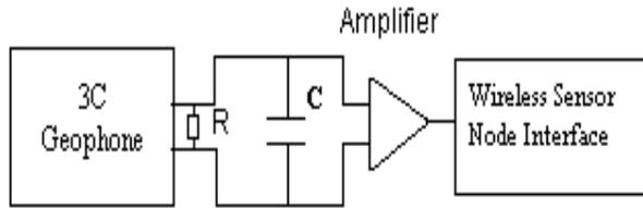
Figure. 3 The geophone circuit. R is the damping resistance. C is the filter capacitor.
