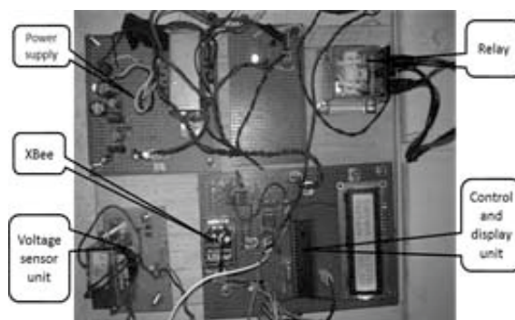
Figure 4: Hardware implementation of intelligent module.
