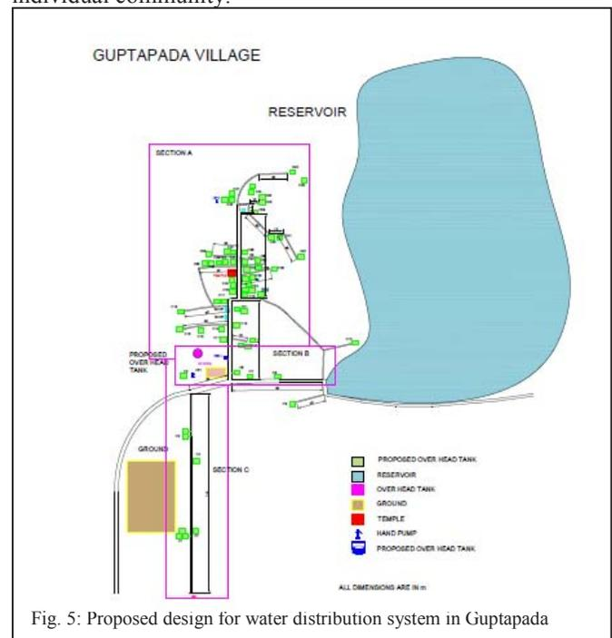
Fig. 5: Proposed design for water distribution system in Guptapada
