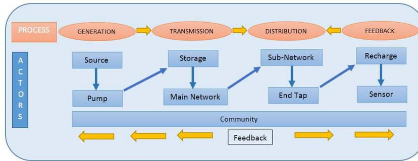
Fig. 2: Water Distribution Scheme as a System
