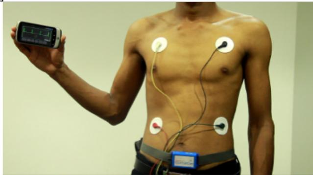
Fig. 3. A patient wearing the Amrita Spandanam ECG sensor device (as a belt). The four body electrodes are connected to the device. The smartphone in the patient's hand shows the live ECG stream as sent from the sensor.
