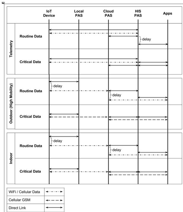
Fig.2. Heterogeneous medium selection and data transmission policy based on the priority of the data and location of the user is summarized in the figure. Note that in many scenarios the data can be stored and send at a later time.
