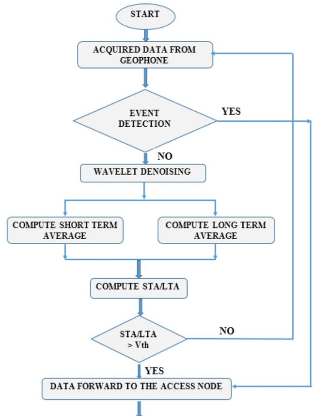
Fig. 3. STA/LTA Algorithm
