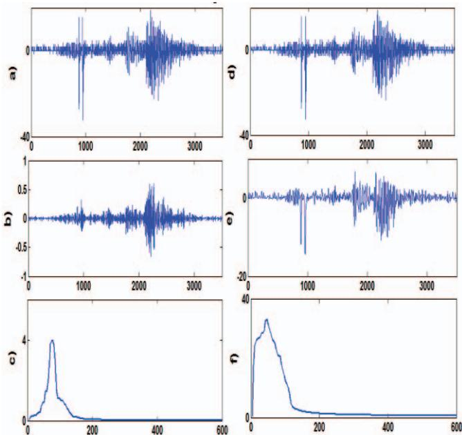
Fig. 7. Vehicular signal (bike), a)-d) Vehicular signal (bike), b) High pass filtered signal, c) fft of Vehicular signal (High pass signal), e) Low pass filtered signal, f)fft of Vehicular signal (Low pass signal)
