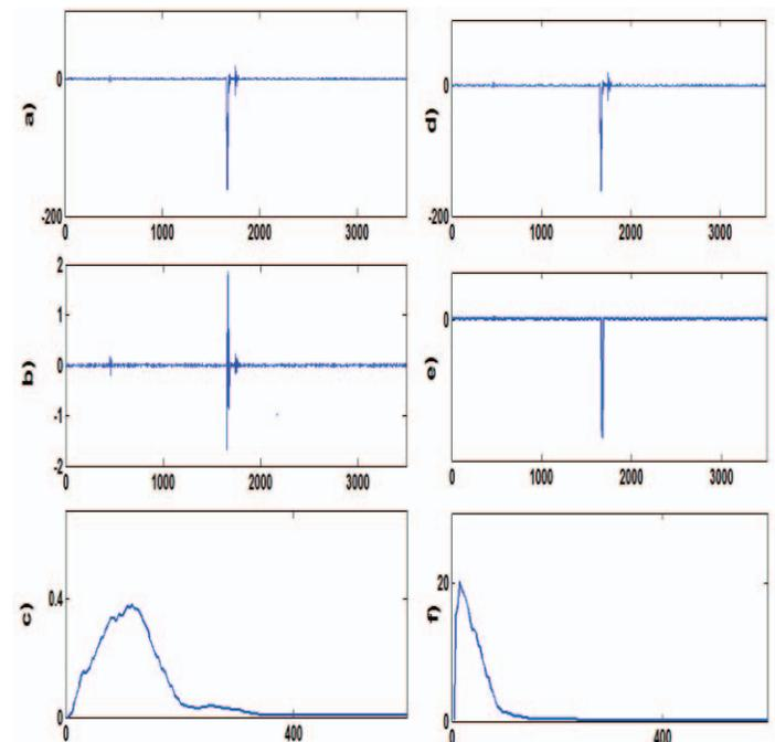
Fig. 6. Weight drop signal, a)-d) Weight drop signal, b) High pass filtered signal, c) fft of Weight drop signal(High pass signal), e) Low pass filtered signal, f) fft of Weight drop signal (Low pass signal)
