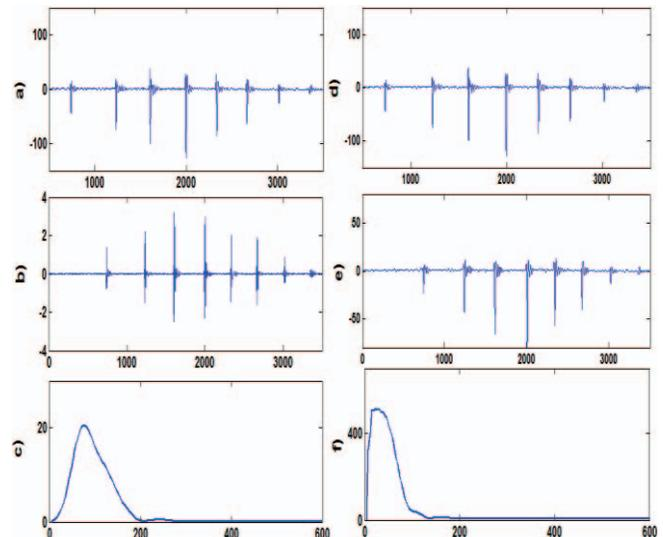
Fig. 5. Footstep signal, a)-d) Footstep signal, b) High pass filtered signal, c) fft of footstep signal(High pass signal), e) Low pass filtered signal, f) fft of footstep signal(Low pass signal)
