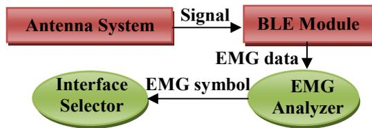
Figure 10. Block diagram of analysis of EMG data
