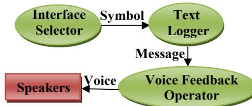
Figure 13. Block diagram of text to speech interface
