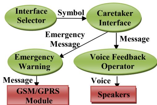
Figure 11. Block diagram of caretaker interface
