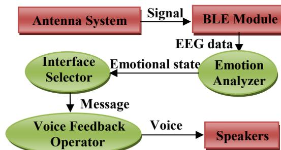
Figure 15. Block diagram of emotion interface
