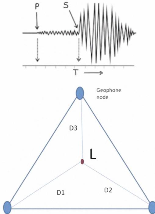
Figure 3: a) Shows the delay in the reception of P waves and S waves. [15] b) Shows geophones placed using Triangulation method. L is the point of origin of the slide and it is distanced D1, D2, D3 from the geophone nodes placed at the edges of the triangle.
