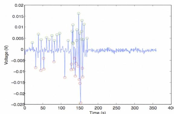
Figure 4 : Data after the peak detection algorithm.
