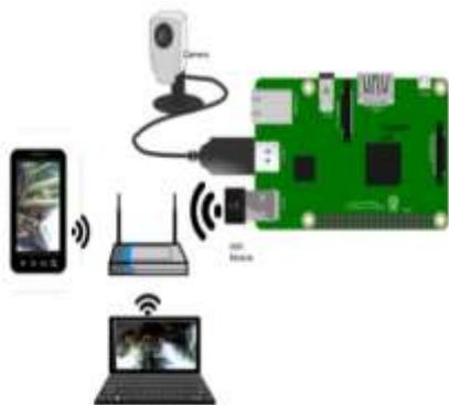
Fig 3. Schematic diagram of video streamer setup
