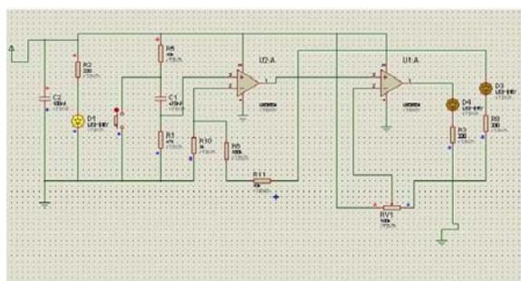
Figure.4. Noise Filtering Circuit
