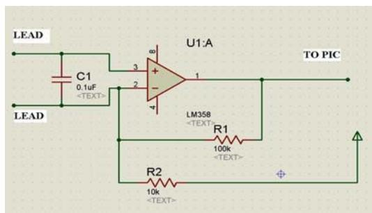
Figure.3. ECG Sensor Circuit
