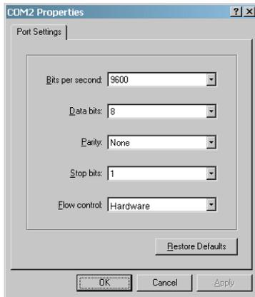
Figure 6. HyperTerminal COM in Properties dialog
