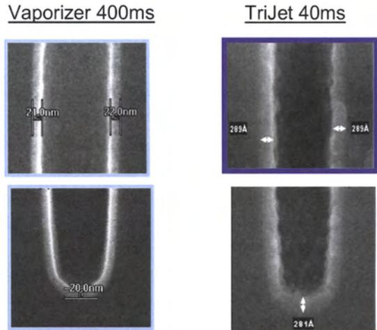
Figure 4 Step coverage results for  $\text{ZrO}_2$  with 40msec using Trijet in comparison to 400msec using a standard vaporizer.
