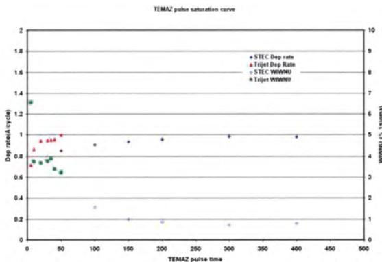
Figure 3 ALD saturation characteristics of TEMAZ using Advanced Vaporizer Trijet compared with previous standard vaporizer.
