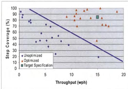
Figure 6. TiN Throughput and step coverage for different processes
