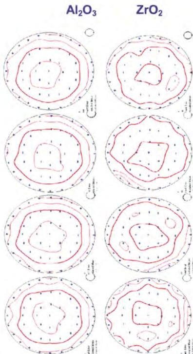
Figure 7 Within Wafer Thickness Non-uniformity for 8 wafers run in Multi Single Wafer System.
