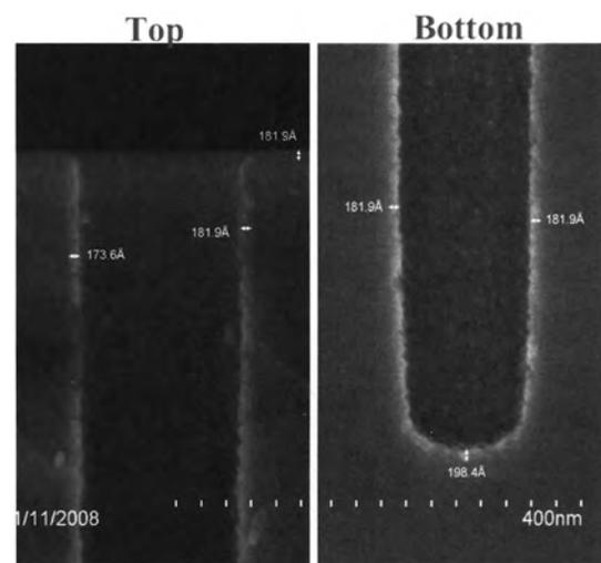
Figure 5 TiN  $\sim 100\%$  conformal coatings on 50:1 high aspect ratio structures. These results were achieved
