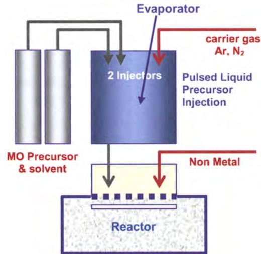
Figure 1 Trijet<sup>®</sup> source has been used for Pulsed CVD (AVD) and ALD. More injectors may be used for multi-element compounds.
