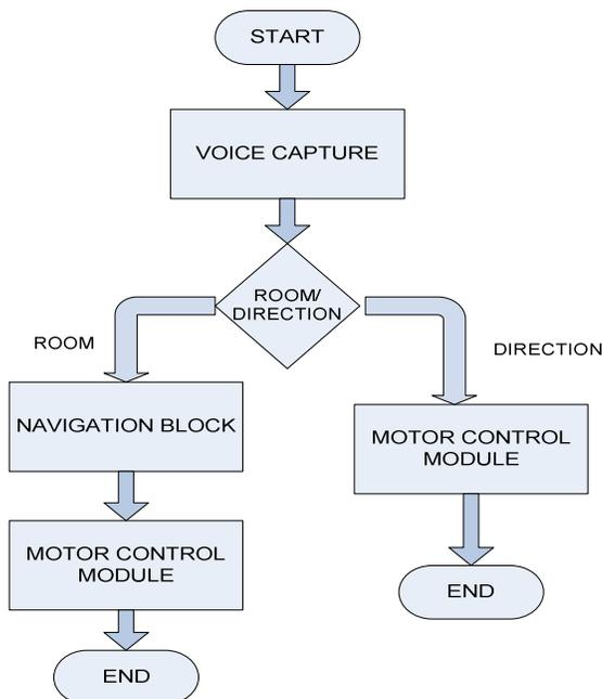
**Figure 2.** Flowchart of the Voice Based Navigation System Algorithm (VNSA)
