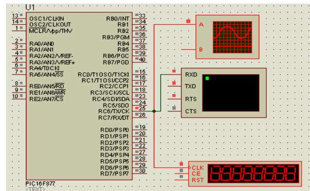
**Figure 7.** Software Simulation of PIC – GPRS Modem direct interface
