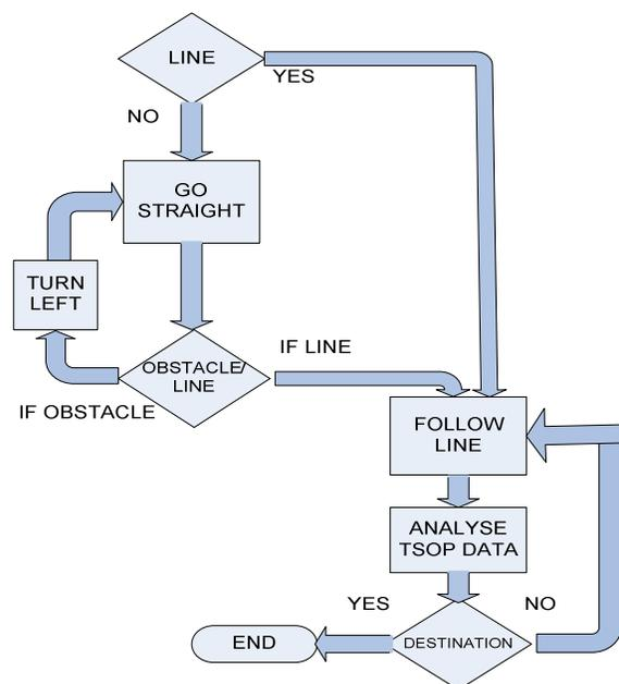
**Figure 3.** Flowchart of Navigation Block which is part of VNSA.
