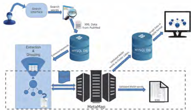
Fig. 1. Architecture of ANeuroNLP frame work. Dataset for this study was generated using the modules included in the rectangular box.
