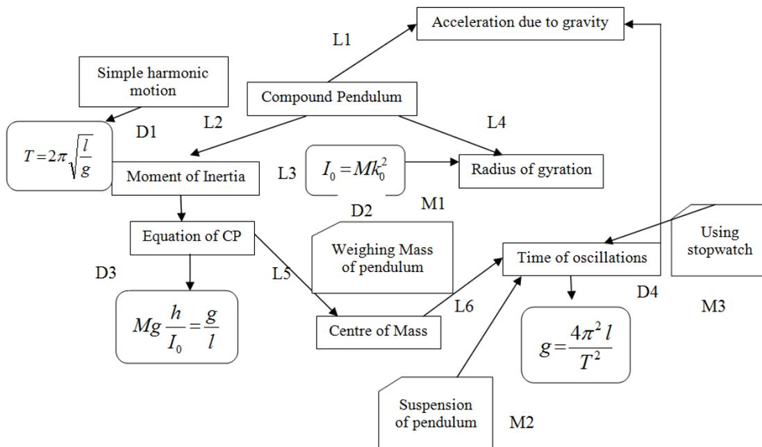
Figure 3: Concept map for Compound Pendulum with n=15 concepts. L-definition/logical deductions, D- Equations used for the experiment, M- Operationalising experiments/modelling procedures.
