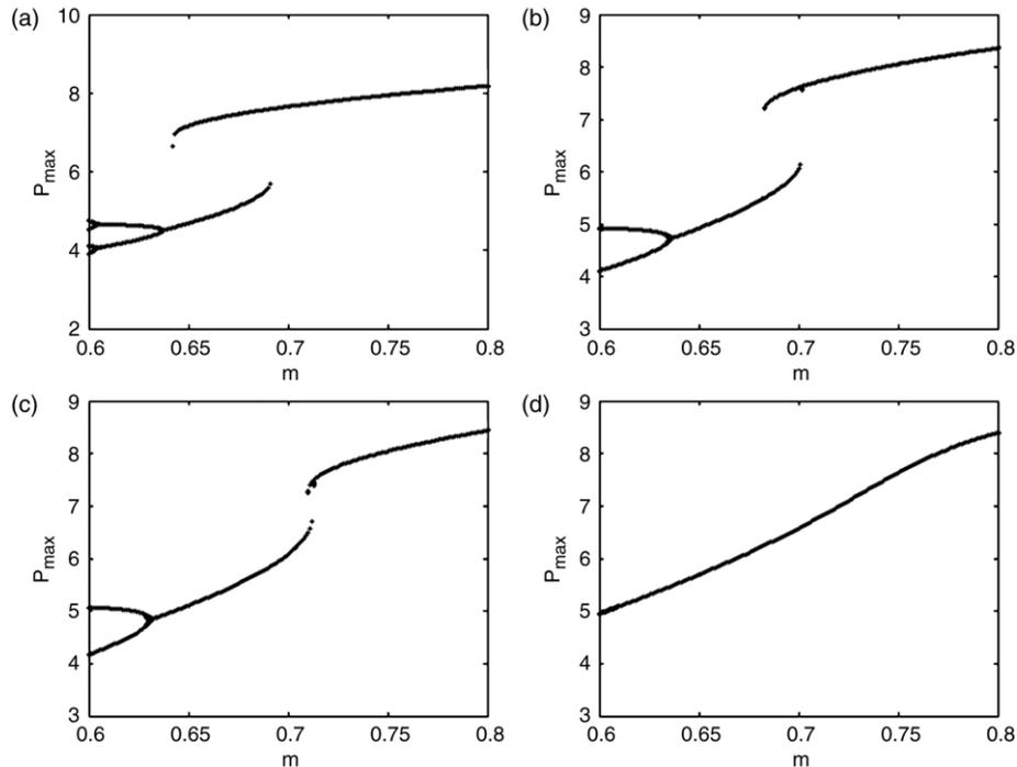
Fig. 11. Variation in the structure of the hysteresis loops with the increase of feedback strength. A positive feedback is considered here. (a)  $C = 0.0003$ , (b)  $C = 0.0015$ , (c)  $C = 0.0024$ , (d)  $C = 0.005$ .
