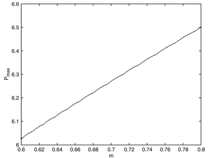
Fig. 7. Variation in the peaks of the normalized photon density of the laser with an increase in modulation strength. A delayed negative feedback is applied to the laser.  $\tau = 0.4$  ns and  $C = -0.005$ . The upper and lower branches of the hysteresis coincide with each other, showing that the bistability has disappeared.
