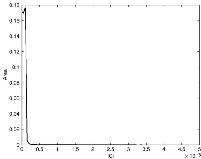
Fig. 6. Variation of the area of hysteresis loop versus the absolute value of feedback strength. Feedback is negative with a delay  $\tau = 0.4$  ns. Notice that the area of the loop becomes almost negligible with a feedback of very low values of feedback strength.
