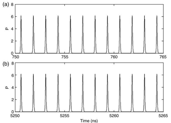
Fig. 8. Time series plots of the normalized photon density of the laser with a delayed negative feedback.  $m = 0.65$ ,  $\tau = 0.4$  ns and  $C = -0.005$ . The pulses obtained while (a) increasing (b) decreasing the modulation strength. The pulses are similar and they correspond to the new dynamical state produced by feedback.
