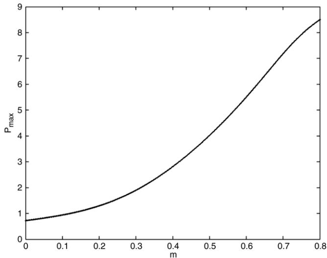
Fig. 12. Bifurcation diagram showing the peaks of the normalized photon density of the laser with an increase in modulation depth. A delayed positive feedback is considered here.  $C = 0.008$  and  $\tau = 0.05$  ns. It is plotted using the continuous time approach. The coincidence of forward and reverse paths shows that the bistability is completely eliminated.
