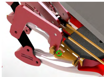
Fig. 2. CAD model of the 3-link serial mechanism for the thumb including flexion, extension, adduction and abduction
