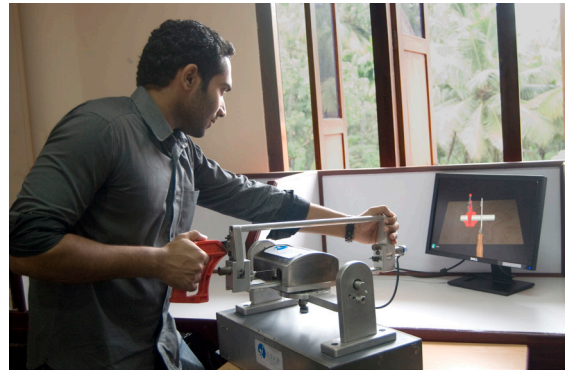
Fig. 1. A novice learning to cut a pipe on the Aptah haptic simulator
