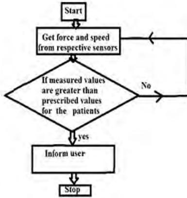
Fig. 2. Flowchart of the control system.
