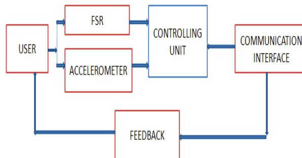
Fig. 1. System architecture of intelligent crutches
