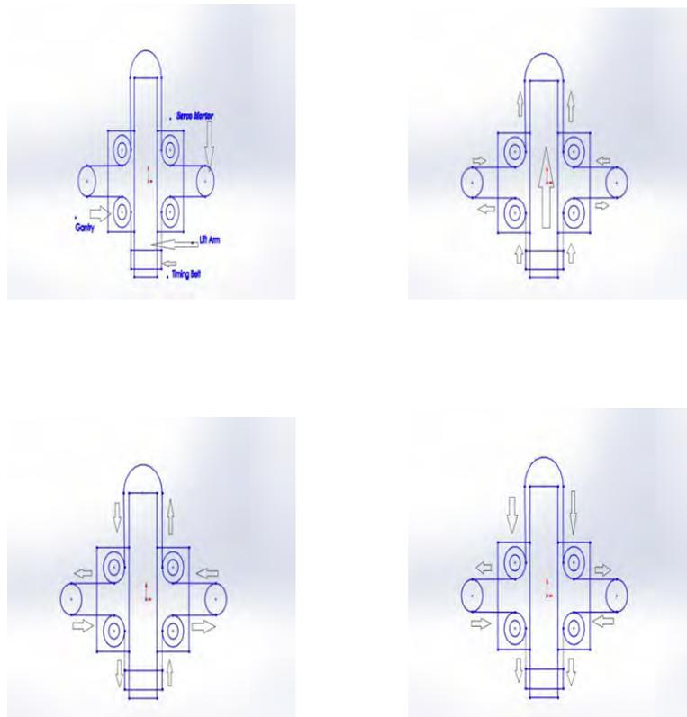
Figure 3: movement of the belt in accordance with the rotations of the motors
