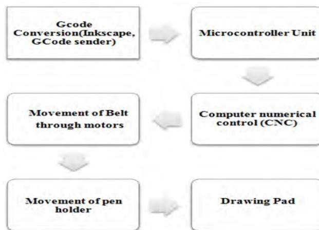
Figure 1: Block diagram of drawing robot
