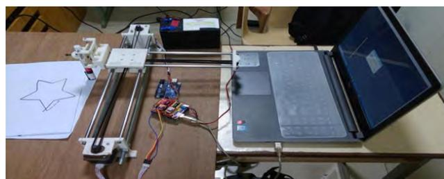
Figure 10: Drawing Robot
