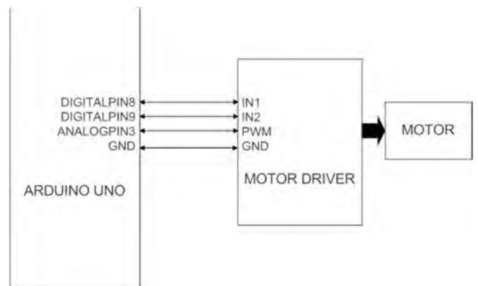
Fig. 5. Port diagram of Arduino Uno and Hercules motor driver
