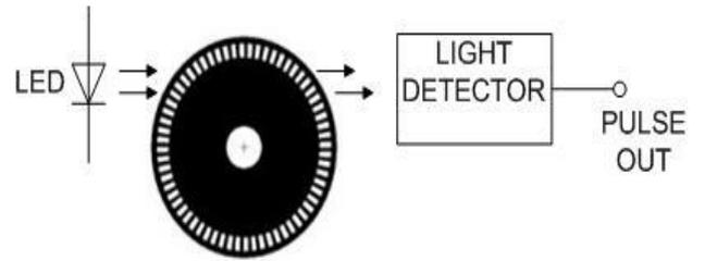
Fig. 3. Schematic of encoder disc placed between led and light detector section of MOC7811
