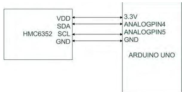
Fig. 4. Port diagram of HMC6352 and Arduino Uno
