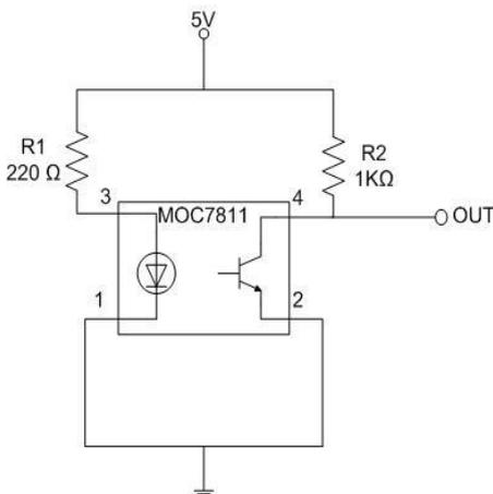
Fig. 2. Circuit diagram for detecting number of pulses using MOC7811 encoder IC
