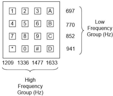
Fig. 2. Mobile Phone Keys and corresponding frequency values
