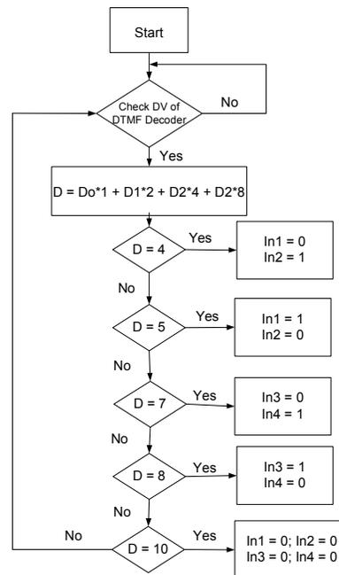
Fig. 6. The MCU Programming Flow Control
