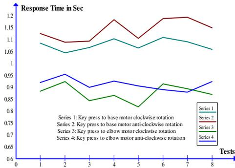
Fig 7. No of test versus response timing plot
