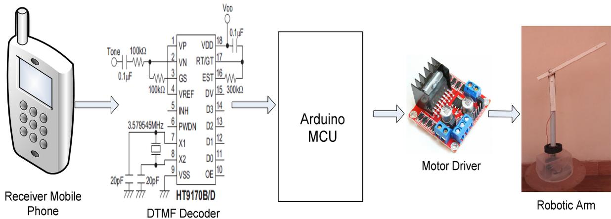
Fig. 5. The Control Diagram with Receiver Mobile Phone
