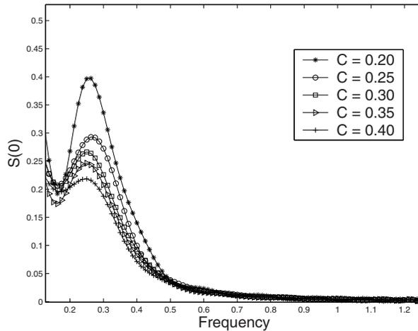
**Figure 5.** The synchronization error decreases with the increase in the frequency of modulation. It can be seen that the modulation frequency is more important than coupling strength in determining the stability of synchronization. Here the amplitude of modulation  $a = 0.1$ .
