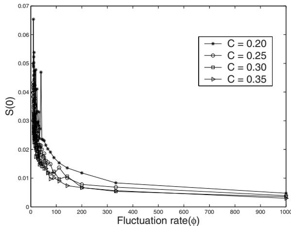
**Figure 3.** The synchronization error decreases with the increase in the fluctuation rate. It can be seen that high coupling could not stabilize synchronization with lower fluctuation rates. Here  $\widetilde{\Delta p} = 0.05$ .
