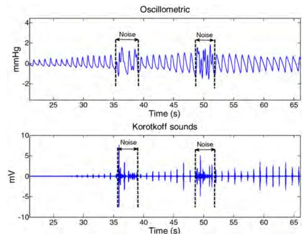
Figure III. A comparison between waveforms of oscillatory auscultatory methods [15]
