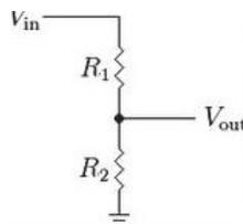
Fig. 2: A simple voltage divider circuit for signal analyzing.
