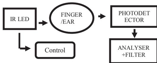
Fig. 1: The proposed Oximeter design block diagram
