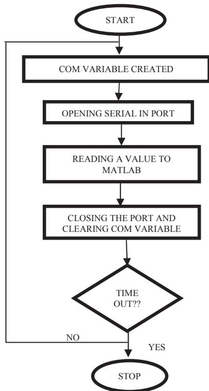
Fig.3: Serial Port and Matlab Interfacing Flowchart
