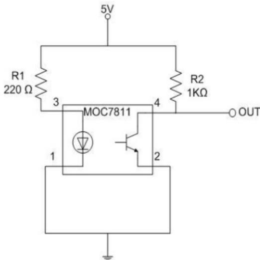
Fig. 4. Circuit Diagram of Rotation Encoder
