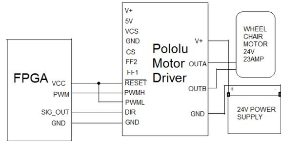
Fig. 5. Port Connections between FPGA, Motor Driver and Motor
