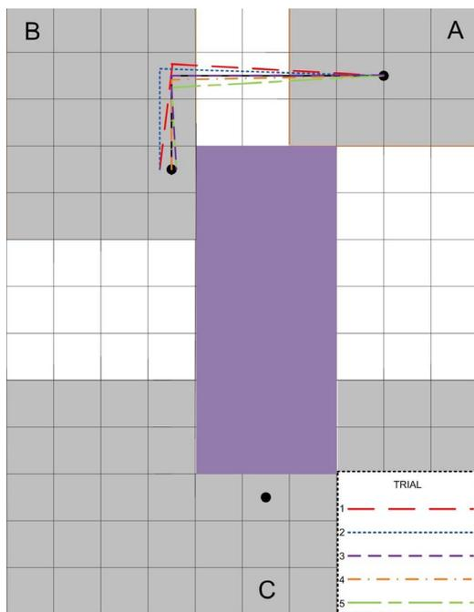
Fig. 7a. Plots showing expected path A to B and different paths obtained for some of the trials
