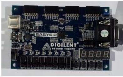
Fig. 2. Digilent Basys 2 FPGA board
