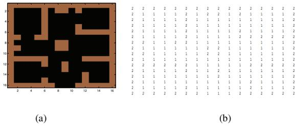
Fig. 3. (a) Sample floor plan (b) Matrix representation of sample floor plan
