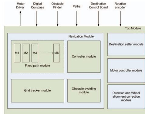
Fig. 2. Block diagram of FPGA controller
