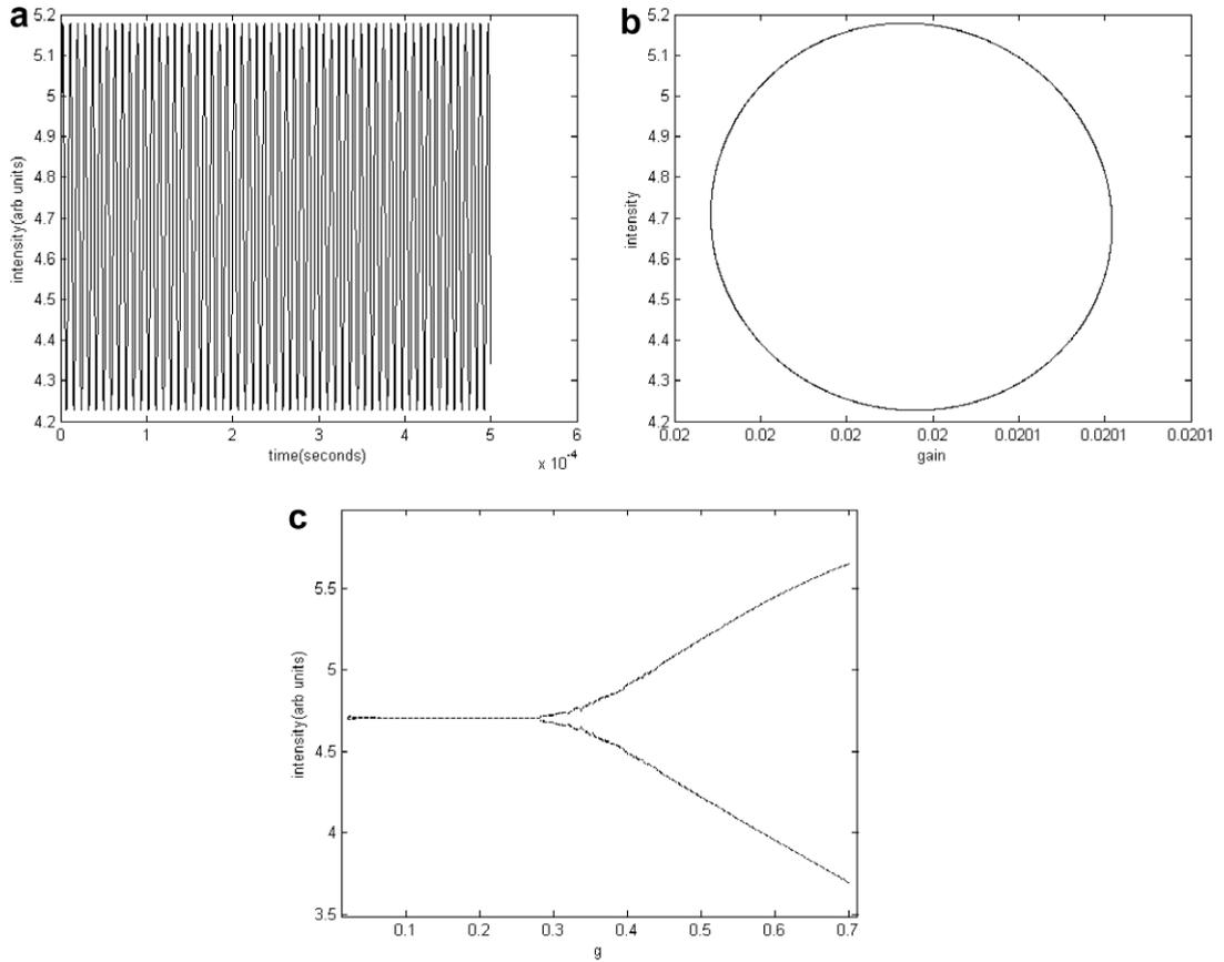
Fig. 5. (a) Intensity time series plot for the laser at  $g=0.5$ . (b) Phase space plot for the laser at  $g=0.5$ . (c) Bifurcation diagram where the maxima and minima of total output intensity is plotted as a function of the control parameter  $g$ .
