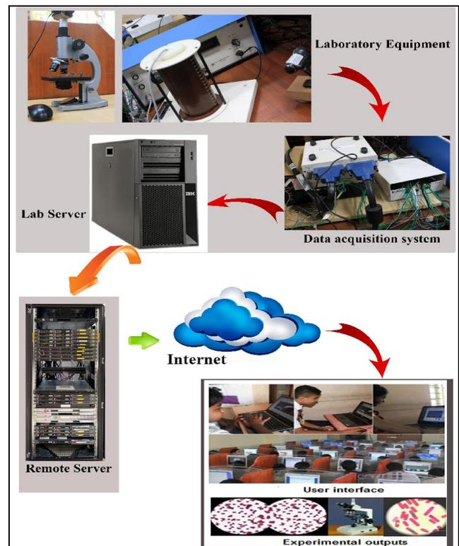
Figure 1. Architecture of remote-triggered virtual lab.
