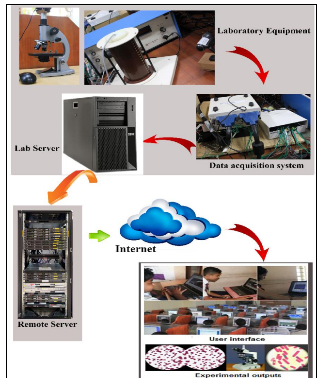
Figure 1. Architecture of remote-triggered virtual lab.
