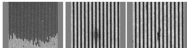
Fig. 2. Defects from Aged Electroplating Baths
