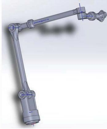
Fig. 2. Design of the 6 DOF robotic arm in Solidworks.
