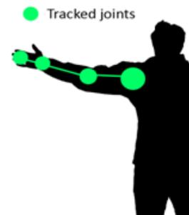
Fig.6 Joints tracked for robotic-arm control
