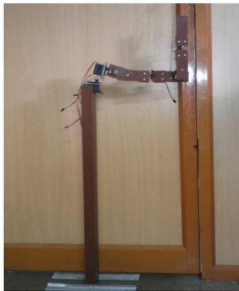
Fig.8 Prototype of the arm to be mounted on the Coco-bot
