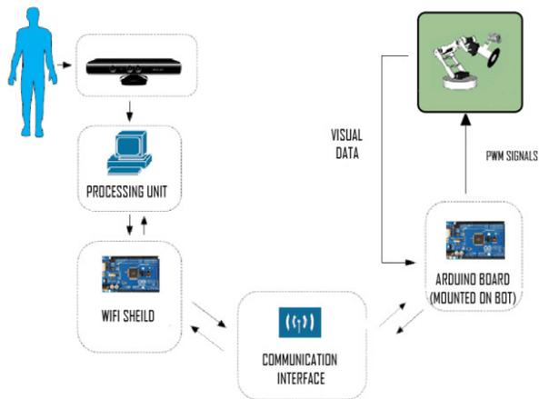
Fig.7. Hexagonal, Wireless Kinect Controller System
