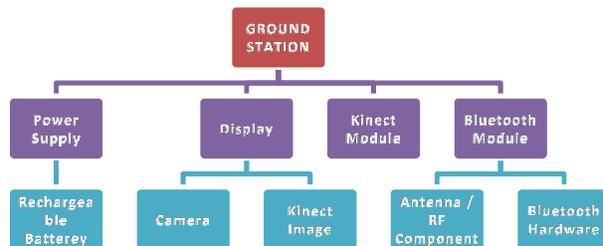
Fig.4 Complete Block Diagram of the Ground Station
