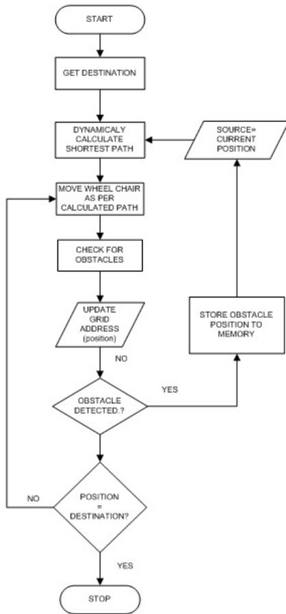
Figure 3. Flowchart of LARN Algorithm
