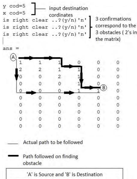
Figure 6. Algorithm testing with three obstacles
