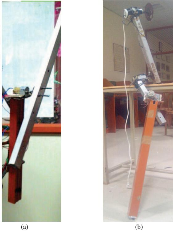
Figure 4 (a) 1 DOF and (b) 2 DOF real time arm
