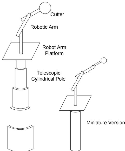
Figure 3. The diagram of robotic arm with cutter and the telescopic cylindrical pole
