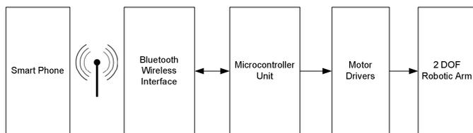
Figure 1. Architectural Diagram of the Proposed System
