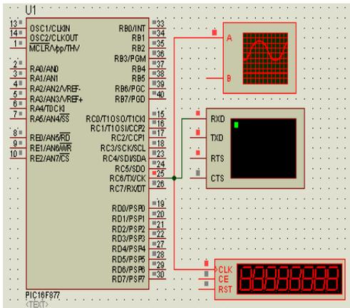
Figure 6. Software Simulation of PIC – GPRS Modem direct interface
