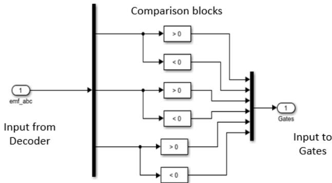
Fig. 10. Comparison logic design for PWM signal selection
