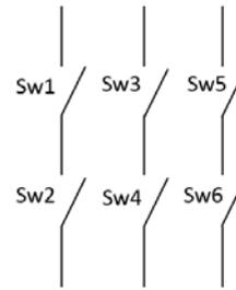
Fig. 5. MOSFET switch arrangement
