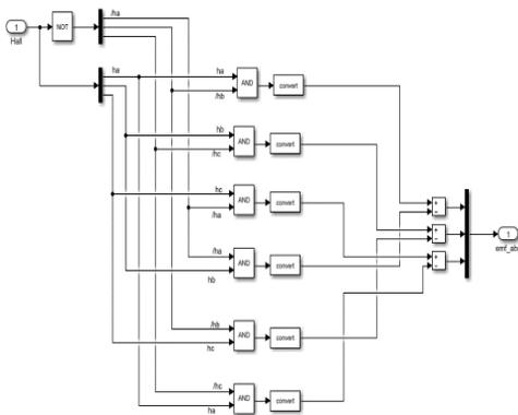
Fig. 9. Decoder block design for computation of Hall sensor input
