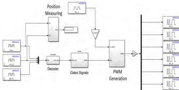
Fig. 8. Speed control Simulink design for BLDC motor
