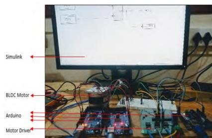
Fig. 15. Hardware test setup
