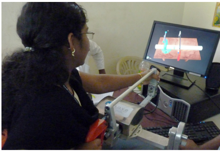
Fig. 7. An industrial training school student cutting a virtual PVC pipe using the SAVE haptic simulator.
