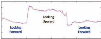
Figure 11. Waveform when eye moves up
