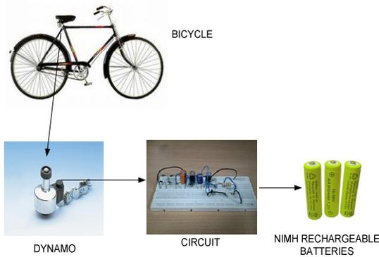
Fig1. Charging NiMH batteries using dynamo
