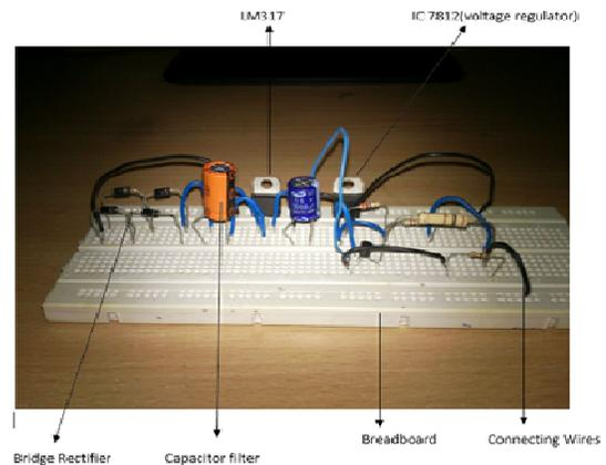
Fig2. Charging circuit
