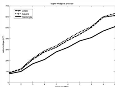
Fig 10. Output voltage Vs Applied Pressure.
