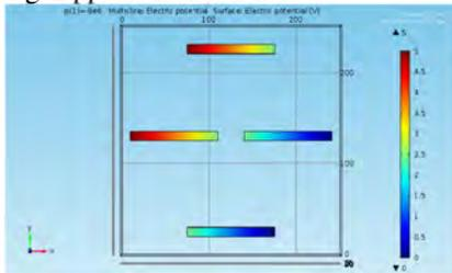
Fig 9. Potential Distribution in a Piezoresistor
