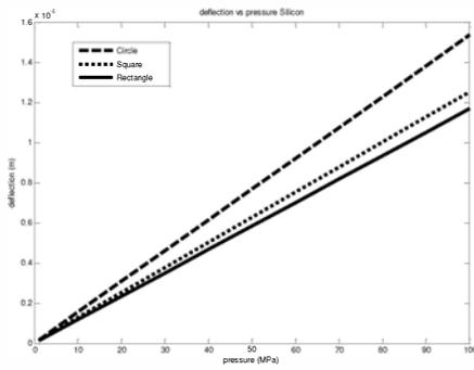
Fig 3. Deflection (m) Vs Pressure(MPa) plot for Silicon diaphragm
