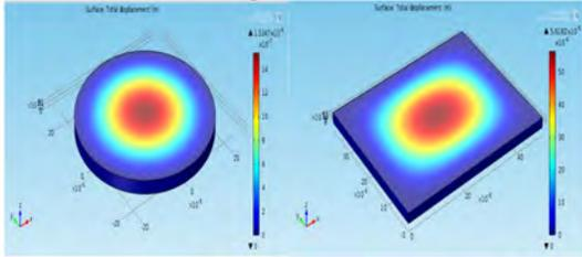
Fig 2. Displacement for Circular and rectangular Diaphragm( $t=30\mu\text{m}$ )
