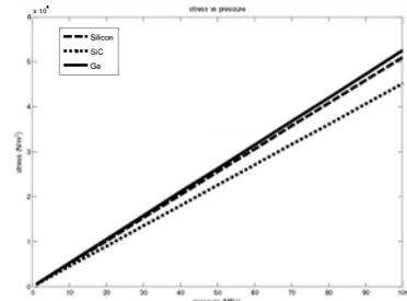
Fig 6. Stress Vs Pressure plot for different materials of Square diaphragm.
