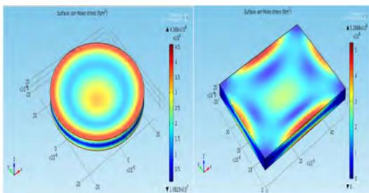
Fig 4. Stress for Circular diaphragm and Rectangular diaphragm( $t=30\mu\text{m}$ )
