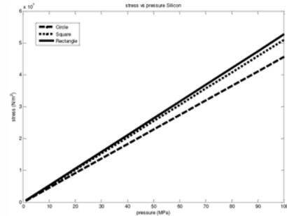
Fig 5. Stress( $\text{N}/\text{m}^2$ ) Vs Pressure(MPa) plot for Silicon diaphragm
