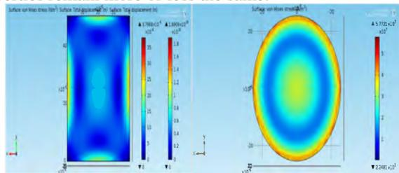
Fig 8. Stress for rectangular and circular with Piezoresistors placed.
